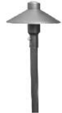
Solid Brass 20" H x 4" W or 20" H x 7" W Nat or Weathered Brass 20W Xenon Bi-Pin (10,000 Hrs.) PVC Stabilizer Stake Includes 25' Lead 18/2 cable Lifetime Includes Polycarbonate De-op lens
